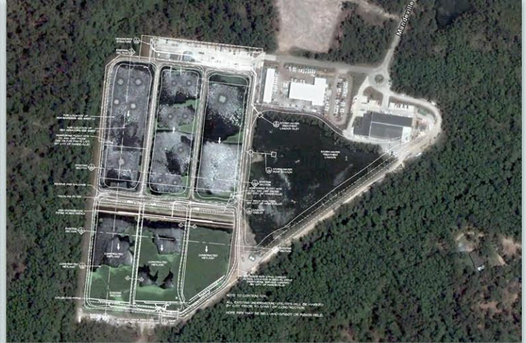
City of Mandeville, LA - Municipal Wastewater Treatment BOD & TSS Effluent and Permit Limit Concentrations Primary Treatment - Aerated Lagoons Secondary Treatment - Sub-surface Flow Wetland with Gravel Trickling Filter Flow Rate - 2 Million Gallons per Day
